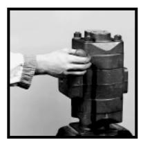
1) Place the pump in a vise with the drive shaft pointIng down. Caution: DO NOT GRIP ON OR NEAR ANY MACHINED SURFACES DURING ASSEMBLY OR DISASSEMBLY. Match-mark all sections. Be sure to align these marks when reassembling.
