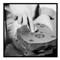
2) If the bushings have been removed, deburr the bushing bores with an emery cloth. Rinse parts in a solvent. Air blast all the parts and wipe with a clean, lintless cloth before starting assembly.
