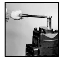
2) Use a socket wrench to remove the 4 cap screws on single units or the 4 hex nuts, studs and washers of multiple units.
