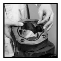
12) Grease the new gasket seals and insert them into the grooves in both sides of all gear housings. Position the first gear housing over the shaft end cover and dowels. Tap it with a soft hammer until it rests tightly against the shaft end cover. Be careful not to pinch the gasket seal. Also be sure that the large rounded core is on the inlet side.
