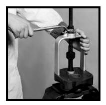
10) Inspect all bushings for scoring or discoloration and replace if necessary. Use a bushing puller as shown in the tool list to remove bushings (see page 4).
