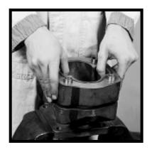
9) Lift or pry off the first section gear housing. Be careful not to damage machined surfaces. Examine and replace if necessary (see page 10).
