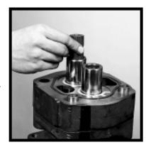
8) Remove the connecting shaft. Remove the thrust plate. Examine and replace if necessary. (See page 10). Remove the driven gear and the integral gear and drive shaft. Keep these together as they are a matched set. Examine and replace if necessary. (\*See page 10). Be careful not to damage the machined surfaces of the gears.
