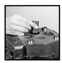
18) Insert the connecting shaft into the spline of the drive gear. Position and place the second gear housing on the bearing carrier as outlined in Step #12. For multiple assemblies
