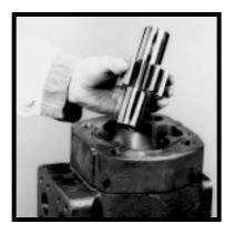
19) Place the thrust plate in the gear housing per Step #14. Insert the drive and driven gears of the second section in their respective bearings. Make certain the gears are in contact with the thrust plate face. Place the port end cover plate in the housing per Step #16. For multiple assemblies
