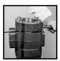
6) Lift the gear housing from the bearing carrier. If prying is necessary, take care not to damage machined surfaces. Examine and replace if necessary. (See page 10)
