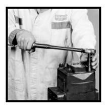
22) Thread the fasteners into the shaft end cover and tighten alternately or cross corner. Rotate the drive shaft with a 6" wrench to check for binding. If there is no internal binding, torque diagonally opposed fasteners to 200 ft. lbs. (2400 in. lbs.); 141 ft. lbs. (1700 in. lbs.) for PGP/ PGM315 models; 450 ft. lbs. (5400 in lbs.) for PGP/ PGM365.
