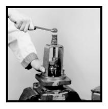
**12)** Use a bearing puller to remove the outboard bearing.
