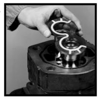
16) Slip the thrust plate with the seal over the gear journals and into the housing bore. The flat side of the seal should face up with the relief groove facing the outlet side. (For single pump assemblies go directly to Step #21).
