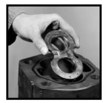
14) Gently slip the thrust plate through the gear housing and into place on the shaft end cover. The channel seal from Step #13 should face the shaft end cover. The relief groove in the plate should face the outlet side of the pump.
