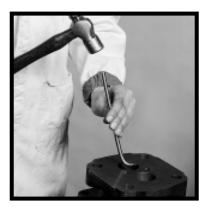
13) Grip the shaft end cover in a vise with the mounting face down. Remove double lip seal by inserting the special seal removal tool (see Tool List) into the notch between the double lip seal and the shaft end cover. Tap the seal out and discard.
