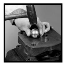
4) New plugs should be screwed in tightly. Stake the plug with a prick punch at both ends of the screwdriver slot and around edges. Peen the edge of the hole 1/32" to 1/16" with a1-1/2" diameter steel ball. NOTE: If new plug or plugs are being installed, coat threads with Loctite™ thread sealant.
