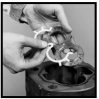
13) Assemble the channel seals into the grooves in the thrust plates with the flat side of the seal facing away from the thrust plate as shown below.
