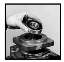
10) If the unit is equipped with an outboard bearing, guide the bearing into its recess in the shaft end cover. This is a light press fit. It may be necessary to lightly tap the bearing into the bore.
