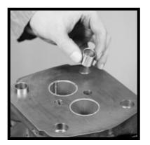
8) See that dowel pins are in place in any new castings. Examine all of the dowels. Before inserting, make certain that the hole is clean and free from burrs. Gently start the pin straight into the hole and tap lightly with a soft hammer.
