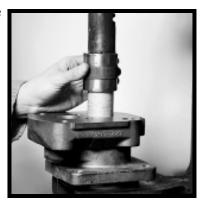
6) Bushings should be pressed into the bores, one at a time, using the special installation tool and an arbor press. Be sure the that the grooves (or seams) are positioned as stated in Step #5. The bushings must be pressed into the bores flush with the casting face. Be sure to support the castings so that they are square and level.
