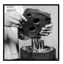
21) Place the port end cover over the gear journals. Align the dowels with the holes in the mating casting. Being careful not to pinch the gasket-seal, tap the port end cover lightly in the center between bearing bores to engage the dowels and to move parts together in the final seating.
