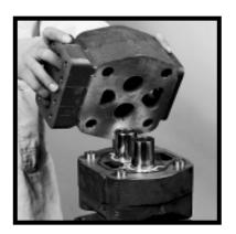
17) Place the bearing carrier onto the journals of the drive and driven gears. Be sure to line up the dowel holes over the dowel pins. When the parts are parallel, squeeze them together or alternately tap over each dowel until the parts are together.
