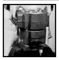
7) Carefully lift or pry off the bearing carrier to prevent damage to contact face and edges. Dowel pins will remain in either the bearing carrier or the gear housing. DO NOT REMOVE THEM.
