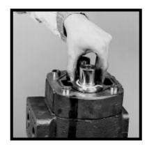
4) Remove the thrust plate. Examine and replace if necessary. See wear guide page 10.
