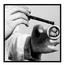
9) Before inserting a new lip seal in the shaft end cover, coat the outer edge of the lip seal and its recess with Permatex Aviation Form-A-Gasket™ No. 3 non-hardening sealant or equivalent. With the metal side of the lip seal up, press it into the mounting flange side of the shaft end cover with an arbor press and bar (see Tool List on page 4). Be careful not to damage the lip of the seal. Press in until flush with the recess. Wipe off excess sealant.
