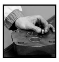
20) Check the plug or plugs in the port end cover to be sure that they are tight. Follow the procedure outlined in Step #4 for new plugs. For multiple assemblies
