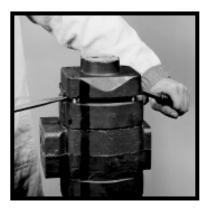
3) Lift off the port end cover. If prying is necessary, be careful not to damage the machined surfaces. Dowel pins will remain in either the port end cover or the gear housing.
