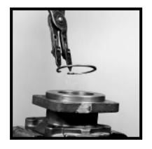
**11)** Install the snap ring in the groove to retain the outboard bearing.
