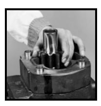
5) Carefully remove the drive and driven gears. Avoid tapping the gear teeth together or against other hardened surfaces. Keep these gears together because they are a matched set. Examine and replace if necessary. (See page 10). Remove the thrust plate from the bearing carrier. Examine and replace if necessary.
