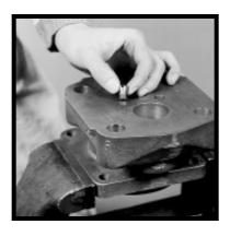
3) Grip shaft end cover in vise with mounting face down. Examine plug or plugs\* to be sure they're tightly in place.
