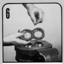
Cut 2 pocket seals 1-1/32" long from the pocket seal strip. Grease these pocket seals and insert into the middle slots in the thrust plate.
