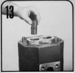
Insert the connecting shaft in the spline of the drive gear.
