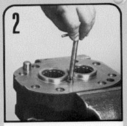
Grip the shaft end cover in the vise with the mounting face down. Examine the plug or 2 check valves, whichever is used, to be sure they are tightly in place. Replace only if parts are damaged or missing. Check valves can be removed with the special tool (see tool list). Screw in new valve with the tool until tight. Peen with a 1%" steel ball to secure.
