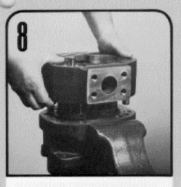
Lift or pry off the first section gear housing. Be careful not to damage machined surfaces. Remove thrust plate as described in step 3.
