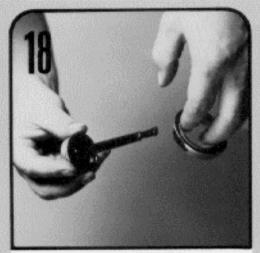
Coat the outside of the seal with Permatex Aviation Form-A-Gasket 3D or equivalent. With the metal side of the seal down, press it into the seal retainer with a 2% diameter bar and an arbor press. Be careful not to damage the lip of the seal.
