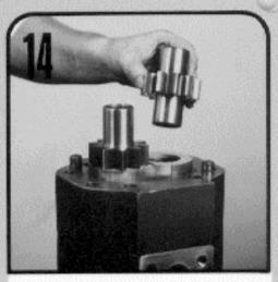
Insert the drive and driven gears of the second section in their respective bearings. Push down tightly against the thrust plate.
