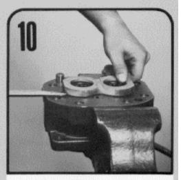
Pry the thrust plate from the shaft end cover, port end cover, or bearing carrier with a screw driver or similar tool. Avoid distorting the thrust plate. Remove and discard all rubber pocket seals and gasket seals.
